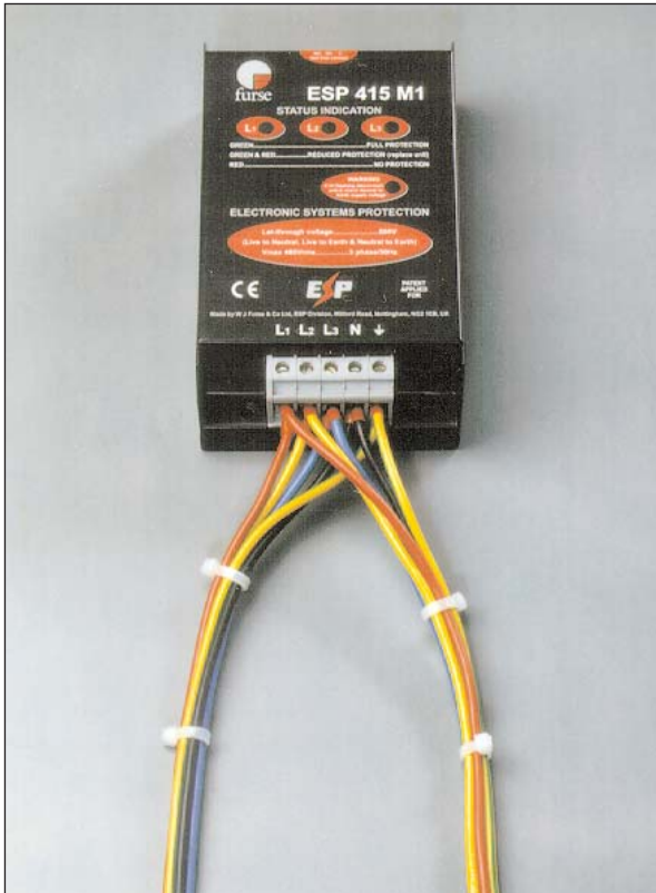
Figure 11 - For connecting leads of up to 50 cm use two sets of conductors (L1, L2, L3, N, \neq ). Each set of conductors has been tightly bound and separated in their routing.
