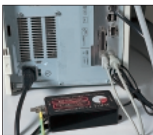
Protector (here an ESP TN/RJ11-6/6) installed on the telephone line connected to a PC's internal modem.
