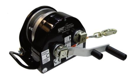
The two speed 100ft winch, is designed specifically for confined space entry/retrieval. Man rated for lowering, raising or supporting personnel. The load can only be moved if the handle is turned, a friction brake is engaged by a weight of 10lbs (4.5 Kg). An inertia brake backs up the triple redundant braking mechanism. The digital counter monitors usage. Mounting brackets available to mount onto the Tripod or Davit
