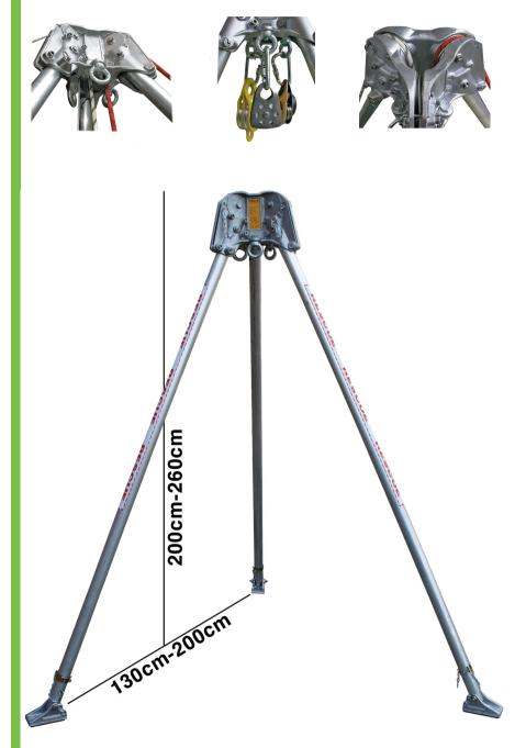
The RT3 has 6 anchor points tested to EN795. The 3 overhead pulleys hold up to 11mm rope. The extra swivel anchor points may be used with pulleys for a double roped rescuer, back-up system, airlines, communication lines, medical kits, tools etc.
