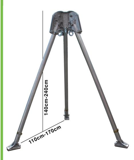
The tripod is the basis of a confined space entry and rescue system giving a strong, stable and portable anchorage point for fall arrest and recovery systems. One worker can carry and erect the sturdy but lightweight aluminium alloy tripod.
