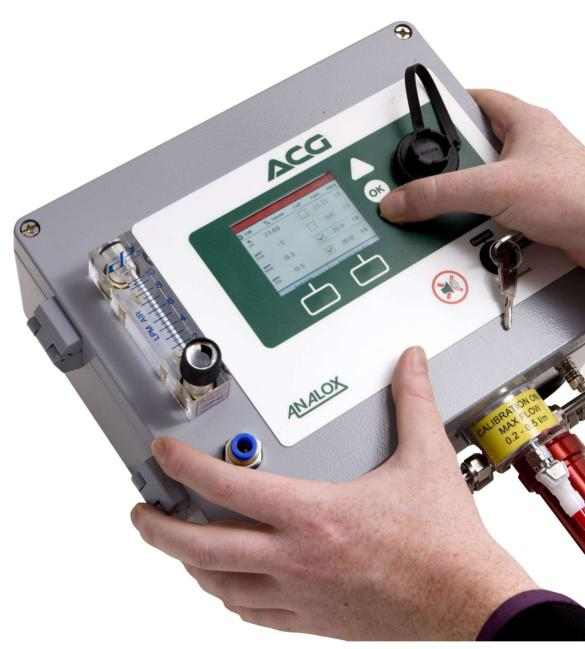
Real time continuous monitoring of contaminants in compressed breathing air
