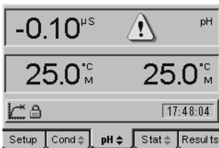
Calibration Reminder Alarm on the pH Channel
