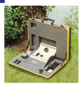
The Model 6035 portable turbidimeter is designed to operate over the range of 0.00 to 199.9 N.T.U. with a resolution of 0.01 or 0.1. Readout is via a 3½ digit LCD. The optical system adopts the proven technique of taking measurements at 90° to the incident light beam. Three glass filters are available to add colour correction, if required.
