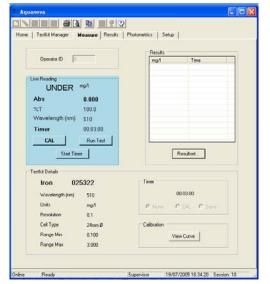
Click on [Run Test], or [Start Timer] if a Save on time out function is included in the method settings.
