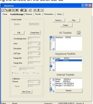
the list of tests available. Use the above procedure to highlight the initial letter and test kit method to up-date the [Testkit Details] in the left hand column.
