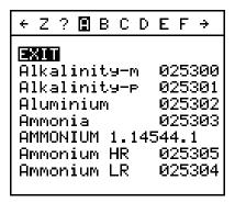
d) Then press the up or down arrow keys to highlight the required test, in the list displayed for the selected initial letter, in the File Select area.
