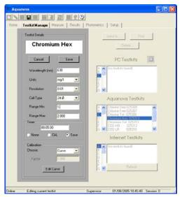
Range Min/Range Max: Click in the box next to either [Range Min] or [Range Max]. You can drag the cursor across one or more digits to highlight them and type in the required digits, or use the delete or backspace keys on the keyboard to delete digits and then type in the corrections.
