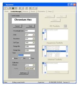
**Calibration:** Click on the down arrow to the right of the box next to [Choose], this will produce a drop down list of the alternative calibration methods.
