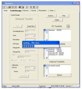
The CD ROM drive should operate. The [Loading...] information box will be displayed showing the progress of loading the test kit methods, this will take longer depending on the number of methods found on the CD ROM.
