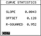
With the [EXIT] option highlighted in the bottom menu bar simply press the enter key to return to the Calibration Curve menu.
