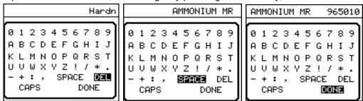
name of the test, including any required part number or id, appears in the top line of the display.
