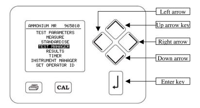
Use the right and left arrow keys to select a digit for adjustment with the up and down arrow
