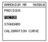
Use the right or left arrow keys to highlight each digit in turn for adjustment with the up or down arrow keys to set the value required.
