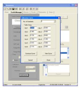
**Curve:** Selecting Curve enables up to six calibration standards to be used to construct and store a calibration curve, enabling test kits with a non-linear response to be used as well as extending the measuring range of other kits into predictable non-linear areas.
