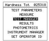
3) Press the down arrow key to highlight [EDIT TEST PARAMETERS] or [CREATE NEW TEST] and press the enter key, the first page of data stored for the selected test or the Default Test when creating a new test, is shown and each option in the list can be edited or set as described in the following paragraphs.
