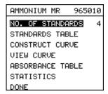
**[NO. OF STANDARDS]** – Simply enter the number of standards that will be used to create the calibration curve, this does not include the absorbance blank. With [NO. OF STANDARDS] highlighted press the enter key. Use the up and down arrows to select from 1 to 6 on the display, with the required number highlighted on the display press the enter key to confirm your selection.
