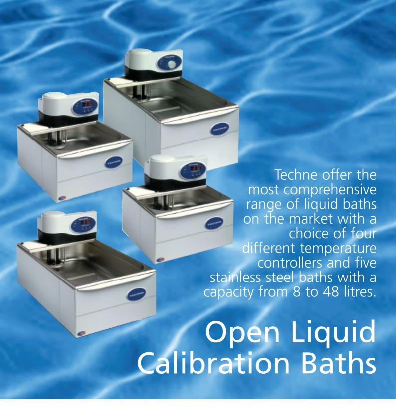
Twenty different combinations of bath offer temperature management over the range of -40  $^{\circ}$ C\* to +200  $^{\circ}$ C to suit most laboratory calibration applications.
