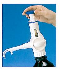
TO DISPENSE, pull the piston up to the top position and eject the set volume by pushing down.
