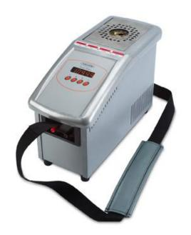
The Tecal 700X Block calibrator utilises a special heater block design giving optimum temperature uniformity and rapid heating rates. The block has 6 fixed bores either metric or imperial sizes with a slim insert matching any of the bores. This block is designed to give unrivalled uniformity across the block but also allow the maximum flexibility between test probe sizes. The block design allows fast heat up and cool down rates and keep the weight of the unit down.
