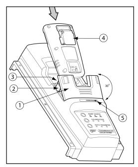
Figure 10. Inserting the GasAlertMicroClip / GasAlertMicroClip XT
