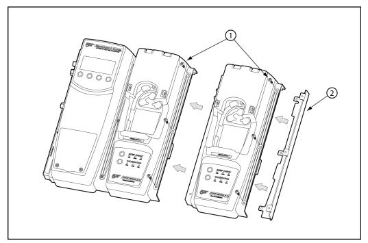
Figure 15. Adding Another Docking Module (Front View)
