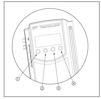
Figure 3. Base Station Pushbuttons
