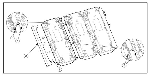
Figure 16. Adding Another Docking Module (Back View)
