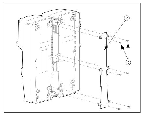
Figure 17. Attaching Back Cover Plate (Back View)
