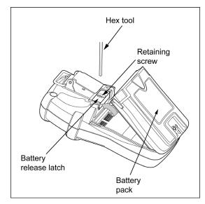
Figure 14. Removing the GasAlertQuattro Battery Pack
