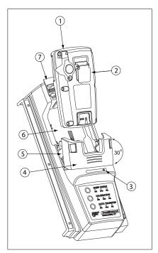
Figure 11. Inserting the GasAlertMax XT / GasAlertMax XT II
