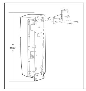
Figure 18. Attaching the Wall Mounting Plate
