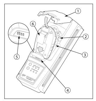
Figure 6. Inserting the GasAlertMicro
