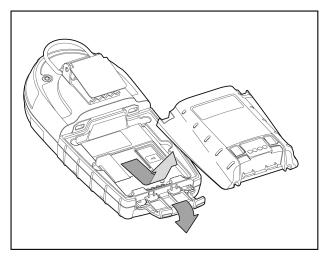
Figure 9. Removing the Micro 5/PID/IR Lithium Battery Pack
