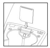
Figure 26. Replacing a MMC/SD Card
