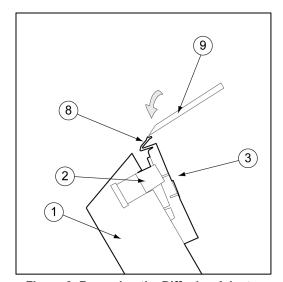
Figure 8. Removing the Diffusion Adapter
