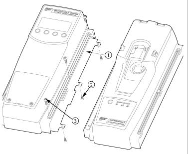
Figure 20. Detaching the GasAlertClip Extreme Module
