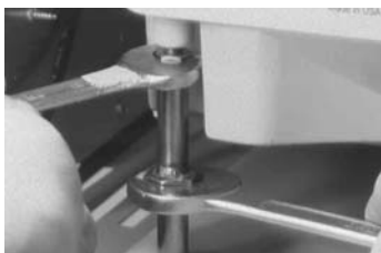
Photo 4.9 - levelling the balance
