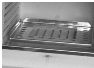
Photo 4.5 inserting the balance pan extension
