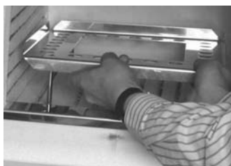
Photo 4.5 inserting the balance pan extension
