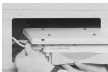
Photo 4.2 - connecting the cables to the balance
