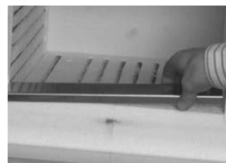
Photo 4.1 - positioning the front brick cover
