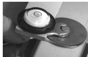
Photo 4.11 - the spirit level; tightening the balance location screws
