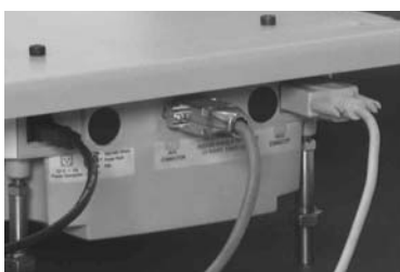
Photo 4.3 - balance cable positions
