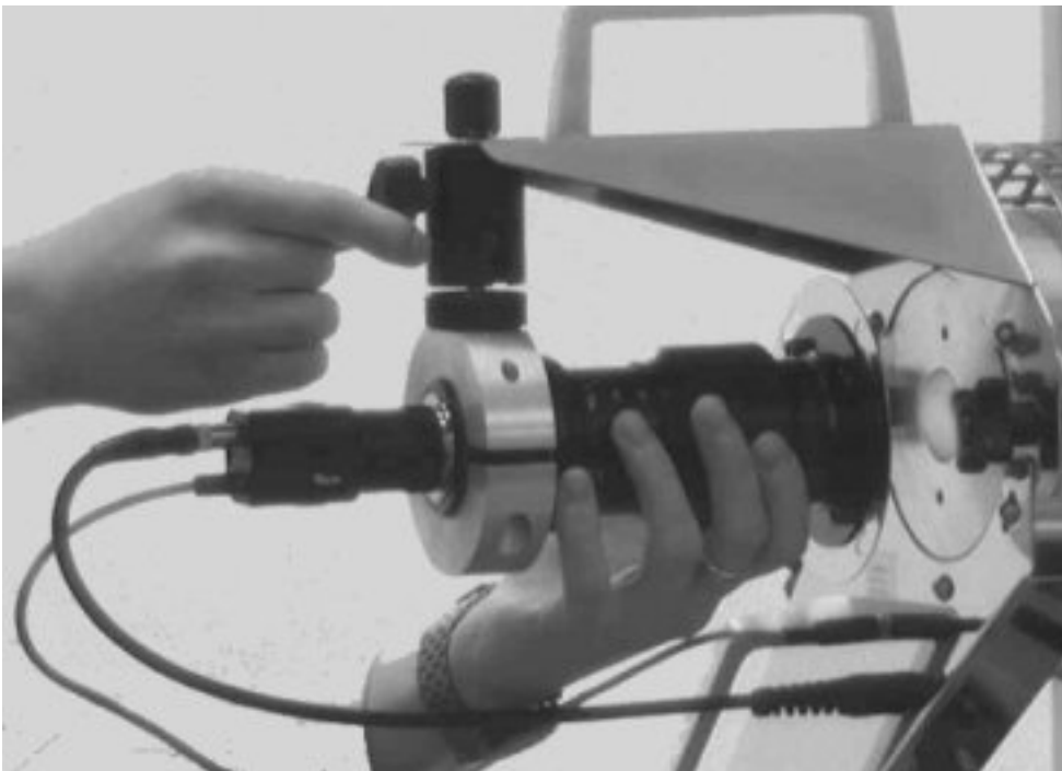
Fig 5m. Adjusting the position of the zoom lens & camera assembly.
