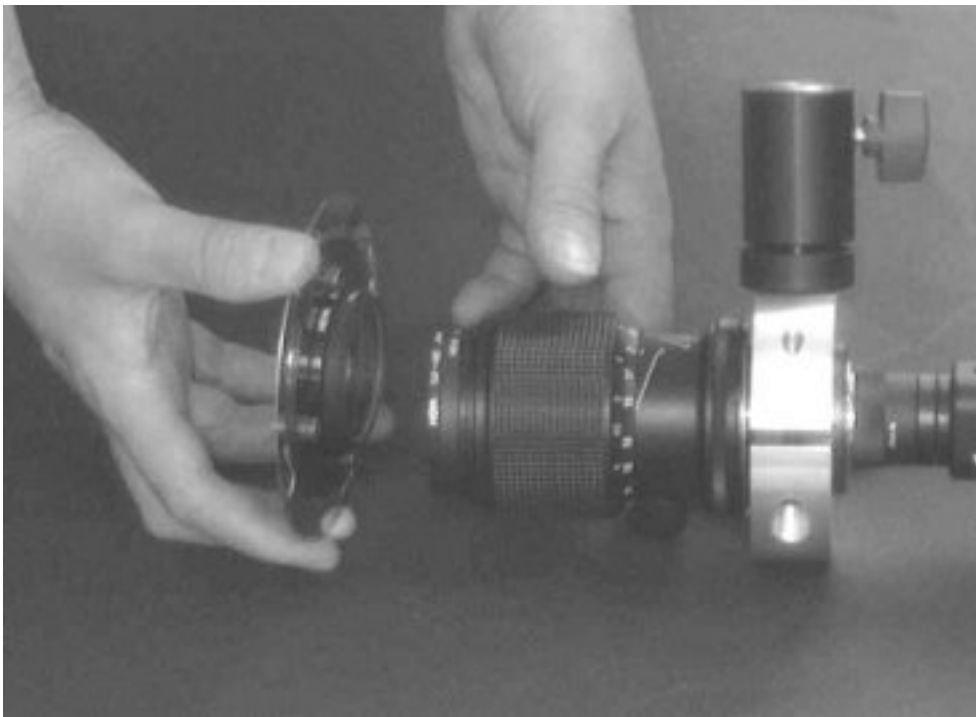
Fig 5j. Mounting the lens heat shield.
