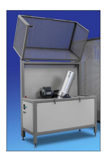
General principles A single tumbler unit is supplied to enable tumble testing to ASTM D 5341-93a.
