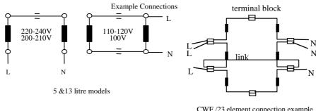
CWF /23 element connection example (1-phase 200-240V)
