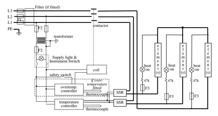
In this configuration the fuses F2 on the supply side of the transformer may be GEC Safeclip, not  $32 \times 6$ mm glass as stated in section 8.1.
