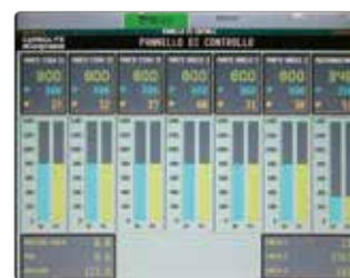
Display showing control zone temperature and setpoint, % power, lance thermocouples, height indicator and wall pressure.
