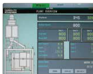
Display showing plant overview with zone temperatures, program, lance thermocouples, height indicator and wall pressure.
