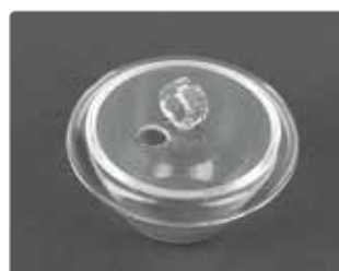
Silica crucible &amp; lid with hole (optional) used for calibration
