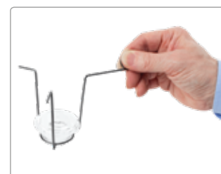
Wire crucible holder (standard) with crucible and lid (optional)
