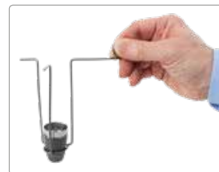
Standard wire crucible holder shown with crucible & lid (VFM/ASTM)
