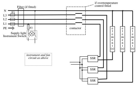
note on 3-phase: depending on EMC filter, there may be 3 neutral wires from the elements to the filter and terminal blocks
