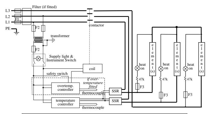
Note: in this configuration the fuses F2 on the supply side of the transformer may be GEC Safeclip, not 32 x 6mm glass as stated in section 8.1.
