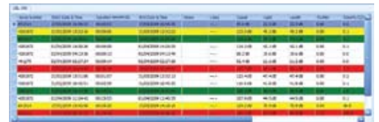
Exposure data can be automatically colour coded according to exceeded action levels
