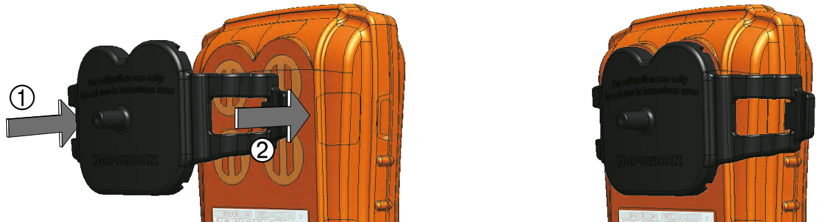
Figure 5: Fitting the calibration/bump test plate
