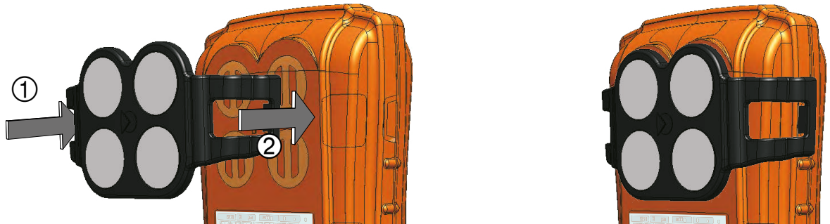
Figure 6: Fitting the external filter plate
