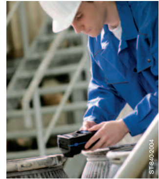
Dräger CMS: Spot measurement at industrial workplaces.
