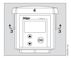
5 Hold the dongle with the "Dräger" logo pointing towards the measuring unit. Then insert the dongle into any of the three slots. Up to three dongles may be installed simultaneously.
