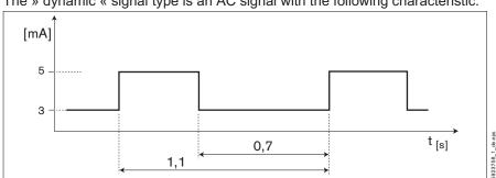
The » dynamic « signal type is an AC signal with the following characteristic:
