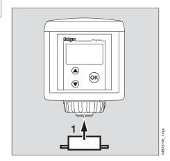
Vent the test gas leaving the adapter into a fume cupboard or into the open air (with a hose connected to the second connector on the calibration adapter).
