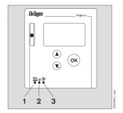
The following icons may be displayed on the right side of the display in measuring mode in order to indicate the operating status of the unit:
