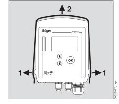
Fit the Polytron 7500 using the metal hooks into the slots provided on the docking station.
