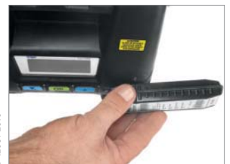
Data Transfer Simply sliding the barcode
