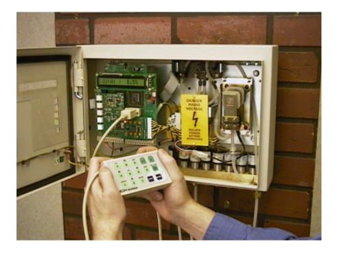
Without the Active-8-or (and key to open the unit), calibration and setup access is impossible, ensuring that there can be no tampering with the system. See the " $CO_2MULTIMONITORINSTALLATION AND SETUP GUIDE" (Part Number 85257) for further information.$
