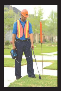
The **GMI** Detecto Pak-Infrared (DP-IR™) is a highly advanced technology capable of detecting methane without false alarming on other gases. The DP-IR is the latest of a new generation of leak survey instruments from **GMI** that will greatly improve the productivity and safety of a walking/mobile survey.
