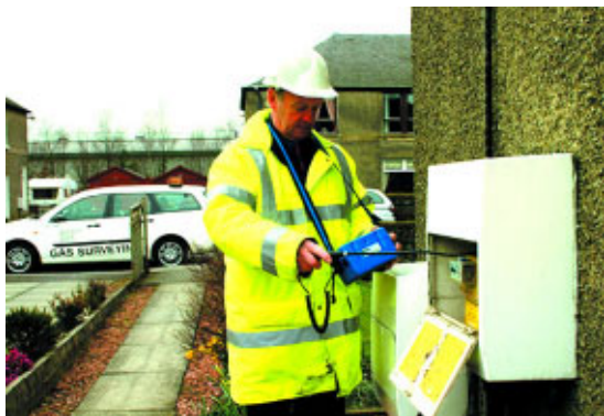
Fig. C-3 Semiconductor Sensor (Flexi) Probe Applications
