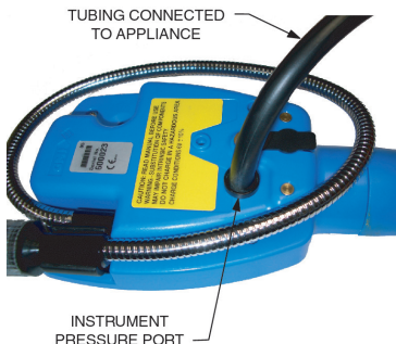
Fig. 10.3 Tubing Connected to Pressure Port
