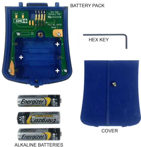
Fig. 4.13 Alkaline Batteries Removed
