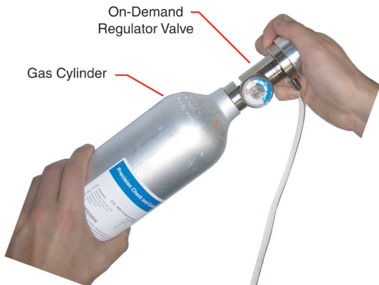
Fig. 2-4 Attach Regulator Valve to Gas Cylinder
