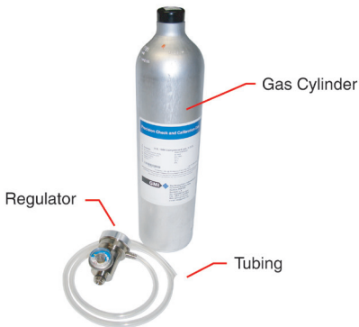
Fig. 2-1 Calibration Gas Setup
