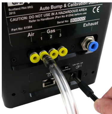
Fig. 2-7 Connect Power Supply to ABC
