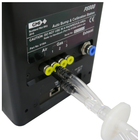
Fig. 2-6 Connect Air Tubing Adaptor to ABC
