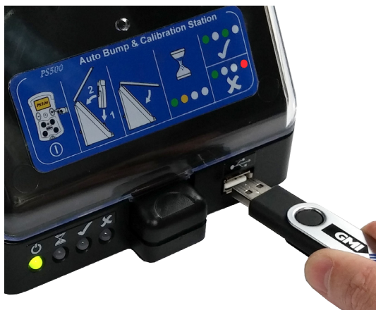
Fig. 5-3 Auto Bump / Calibration Station USB Port
