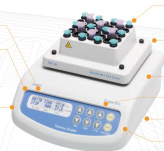
Convenient interchangeable block for 20 or 12 microtubes provides flexibility for an easy change in application
