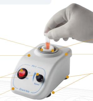
In 'touch' mode, agitation starts in response to pressure on the pressure sensitive cup
