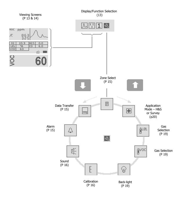
From the DISPLAY/FUNCTION selection screen, highlight the function menu icon then press ENTER. Use the UP/DOWN keys to view the available functions, then press ENTER to select the function options.
