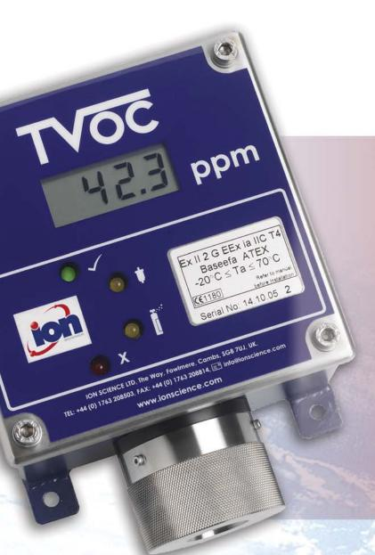
**TVoc** is the first Intrinsically Safe, fixed photoionisation detector (PID) of its kind for continuous detection and measurement of total volatile organic compounds (VOCs). With a 4-20 mA analogue output **TVoc** can be integrated into a DCS control system to give warning or control of high VOC levels in the working environment.
