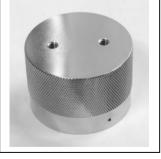
If a unit is to be placed in an inaccessible or difficult to reach location TVOC can be fitted with a Fixed bump adaptor, part number 849217 to enable remote bump testing. This enables the unit to work as a diffusive instrument but allows a bump gas to be applied. This again would replace the standard sensor cap and looks as follows:
