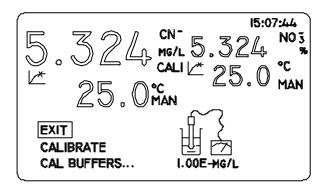
An icon will appear the CAL 1 buffer value and the first part of the calibration. The display will also indicate CAL 1 to the right hand side of the main reading. The buffer values can be changed at this point by entering the CAL BUFFERS... menu and setting new values by using the numeric keys and pressing .
