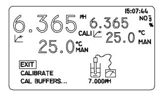
An icon will appear indicating the CAL 1 buffer value and the first part of the calibration. The buffer value(s) can be changed at this point by entering the CAL BUFFERS... menu and setting new values by using the numeric keys and pressing .
