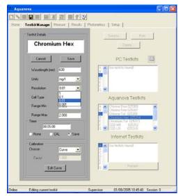
**Resolution:** Click on the down arrow to the right of the box next to [Resolution], this will produce a drop down list of the available Resolution options.
