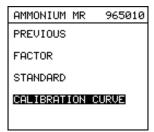
A list of seven options is displayed. The top three must be completed to create a calibration curve, the following three return information and statistics useful in verifying the curve, finally select [DONE] to save the test kit method and return to the main menu.
