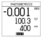
The photometrics measurement screen is displayed, this shows the absorbance value at the top followed by the transmittance value and then the selected wavelength. The absorbance and transmittance values displayed are continuous live readings at the wavelength displayed. Measurements may be made using the following procedure.
