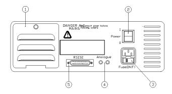
1. Lamp Access Panel allows the user to gain access to the tungsten halogen
