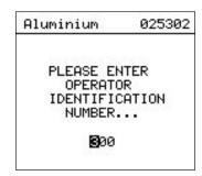
Scroll down the main menu to [SELECT OPERATOR ID] using the arrow keys and then press the Enter key.
