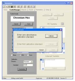
**Standard:** Selecting Standard enables a single standard solution to be used for calibration along with the blank, effectively storing a straight line calibration curve based on these two points.
