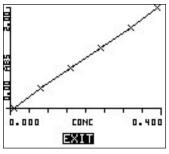
Select [TEST PARAMETERS] from the main menu using the arrow keys and then press the Enter key. This option allows the user to view the currently loaded test parameters. If the test uses a Calibration Curve and not a Factor, the display will show an option to view the curve. This can be selected by highlighting [VIEW CURVE] and then pressing the Enter key.
