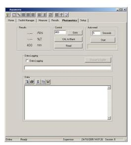
The Photometrics screen displays the live reading from the instrument.
