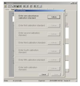
[Enter zero absorbance calibration standard] performs a calibration on the instrument.
