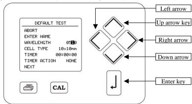
keys, press the enter key to confirm the setting when ALL digits have been correctly set.
