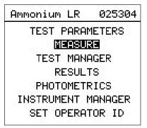
(Should you wish to view the specific settings for this method press the up arrow key to highlight [TEST PARAMETERS] then press the enter key.)
