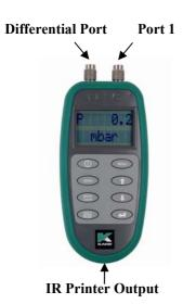
Always use the top right hand port (Port 1) for taking single channel measurements (pressure or vacuum). Only use the left hand port for differential measurements.
