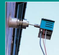
KM9108 Gas Conditioning Unit
