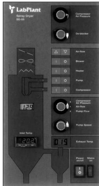
Control panel : A combination of touch sensitive push button switches and rotary dials ensures accurate control and repeatability.
