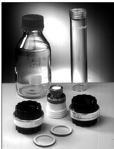
Sample Collection Bottle, Collection Tube, SVL Connectors with PTFE Seals and Counter Current Adaptor.
