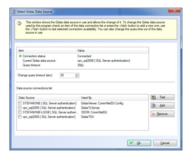
This window shows the *Gidas data source* in use and allows the change of it. To modify the data source used by the program select one element from the list of available data sources or press the
