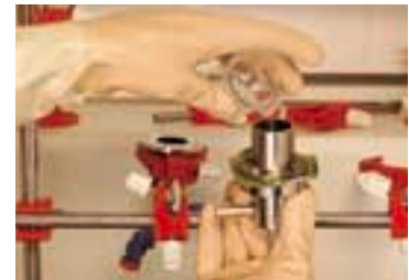
In laboratory tests the permeation times of chemicals are determined. The Vautex Elite resists even toluene, 96% sulfuric acid, chlorine or ammonia for over 8 hours and in almost every case reaches the highest standard class.
