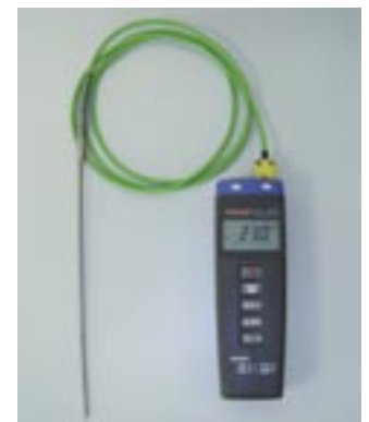
Temperature gauge for RAKU 100, easy to operate, NiCr-Ni temperature sensor, display range 20 – 1200 °C, optional connection of second sensor with display changeover
