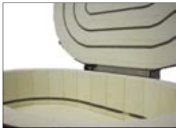
Kiln interior with circular lower side heating
