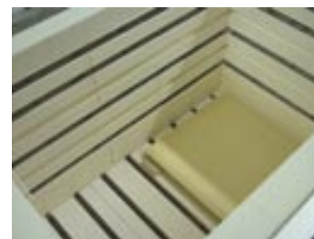
Firing chamber with heating from 5 sides
