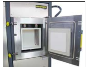
Chamber made of ceramic fiber
