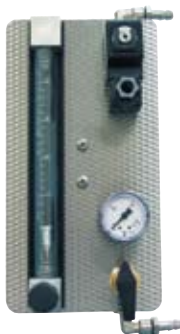
Gas supply panel for nonflammable protective gas with shutoff valve and flow meter with regulator valve, piped and ready to connect
