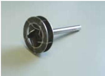
Ventilator in rear wall of furnace
