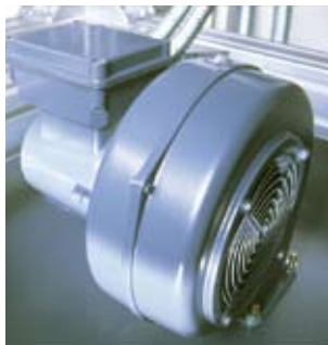
Cooling fan connected to automatic vent flap for shorter cooling time
