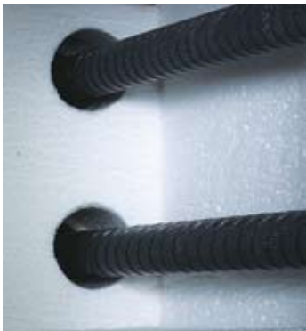
Furnace chamber with high-quality fibre material and SiC heating rods in the sides of the furnace
