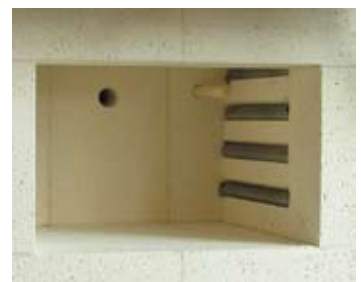
Furnace interior with high-quality lightweight refractory brick insulation
