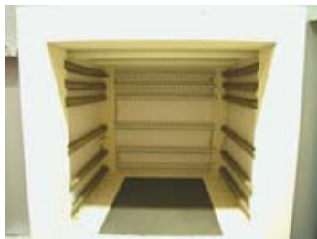
Interior of low heat storage fibre material for fast cooling times in LF models
