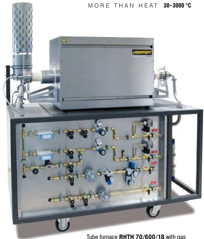
Tube furnace RHTH 70/600/18 with gas supply system 4
