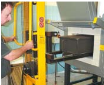
Working with protective gas boxes for a protective gas atmosphere using a loading carriage
