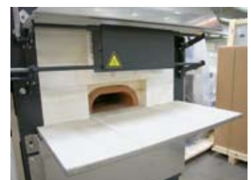
Work platform in front of muffle to place load
