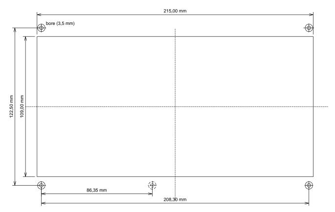
The front panels have a total size of 243 x 149 mm. The front panels project from the cut-out at top and bottom by 20 mm, left and right by 14 mm.
