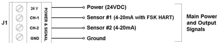
Figure A - 6 Power and Signal Connector J1 on HART Supported TRANS-2
