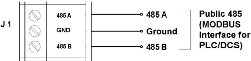
Figure 4-9 Wiring Diagram for the ModBus Interface
