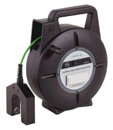
The 715 Portable uses a range of infrared sensors to make the sludge interface detection. Infrared attenuation has been selected as it is ideally suited to detecting the sludge present in the interface zone. This tends to be considerably 'thinner' than the sludge that is present at the bottom of a settlement tank
