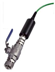
The IL55BV2 Sensor is intended for in-line measurement of solids in water. It uses Infrared Light at 960nm and operates using the Back-Scatter Principle. The light is transmitted and received through a lens that is optically split.
