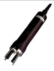
The Turbi-Tech 2000LA Sensor uses Infrared Light at 860 nm and operates using the Light Attenuation Principle. The optics are housed in cylindrical glass tubes that are moved past a set of polyurethane wipers seals to carry out the cleaning process. The cleaning mechanism is then sealed by 2 Nitrile 'H' Rings that finish the cleaning process. The Nitrile seals can be exchanged for Viton if the process media dictates.
